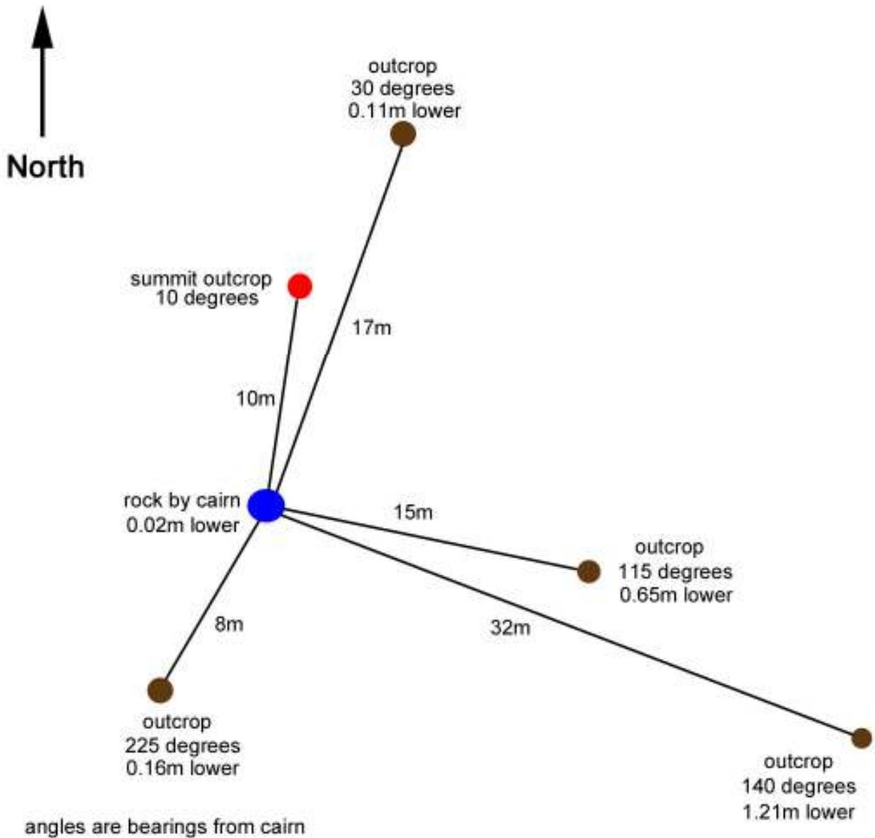
The summit position was identified as a rock outcrop 10m distant from the cairn and at a bearing of 10 degrees from it. The highest rock under the cairn was 0.02m lower. All other candidates were measured to be greater than 0.1m lower.
