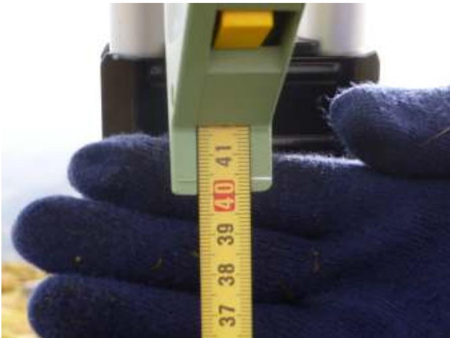
**Measuring the offset, 0.404m, for the Leica Viva GS15 on the summit**
