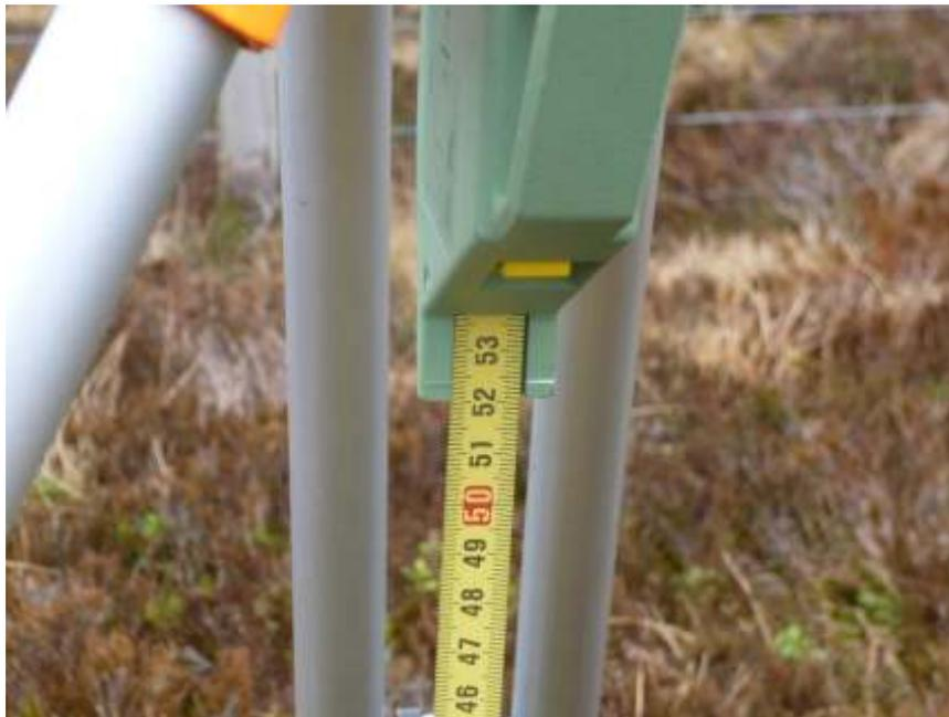
**Measuring the offset for the Leica Viva GS15 on the summit of Corwharn**
