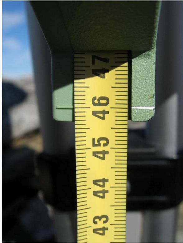
**Measuring the offset for the Leica Viva GS15 on the summit of Little Wyvis**
