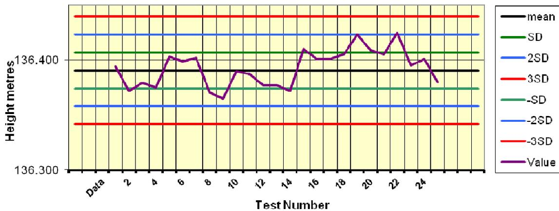
In addition, we check the instrument periodically by taking measurements on an Ordnance Survey Fundamental Bench Mark, processing the data and comparing it with the OS derived values. Height should agree within about 0.05m. The latest two measurements are given in the table below.
